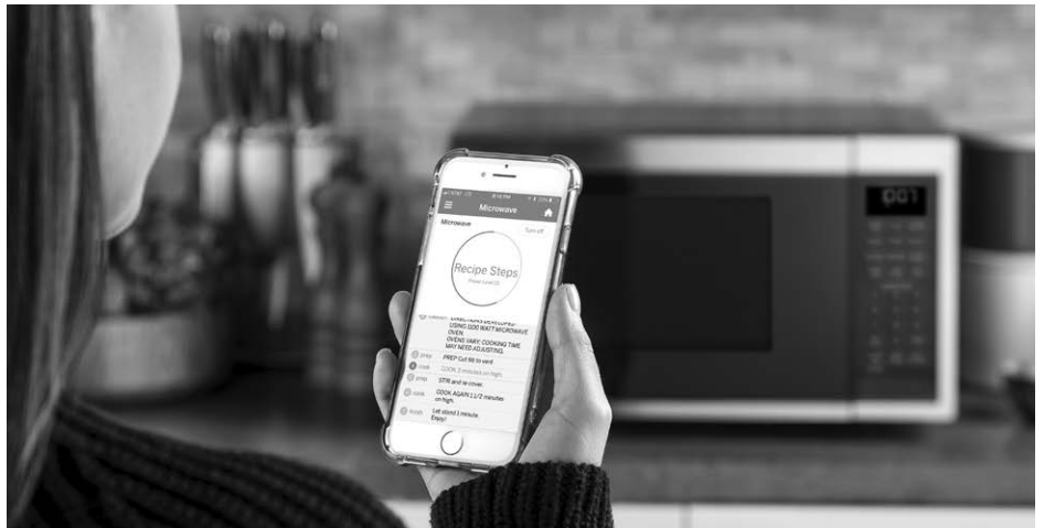
Smart microwave ovens, such as the GE model shown here, include barcode scanning technology to allow product-specific cooking instructions to be sent to the appliance. Photo credit: GE
